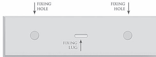
GUTTER STRIP – 1200mm in length
